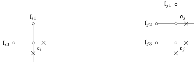
(a) Layout I: c_j = l_{j1} \vee \bar{l}_{j3} (b) Layout II: c_j = o_j \vee \bar{l}_{j3} = (l_{j1} \vee \bar{l}_{j2}) \vee \bar{l}_{j3}
