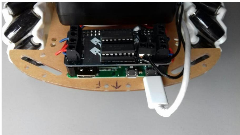
In the photo above, you will just be able to make out the terminal numbers for motor 1 and motor 2 to the left of the MotoZero. These are in turn connected to motors 1 and 2 respectively on the right hand side of the robot car (facing forward).
