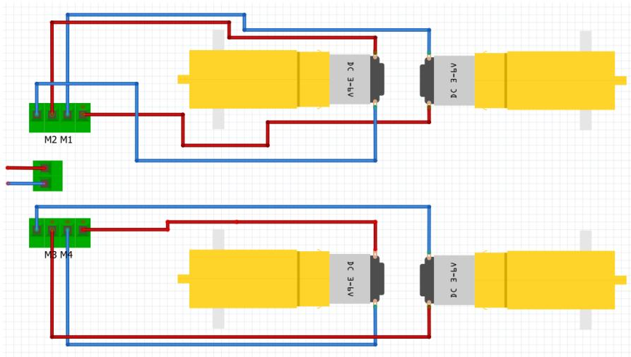
The diagram above is a simple representation of how the motors are wired to the MotoZero. The MotoZero sits on top of the RPZ, and the 40 MotoZero sockets fit exactly onto the 40 RPZ GPIO pins. The green terminals to the left hand side of the diagram represent the terminals that are present on the MotoZero motor controller.
