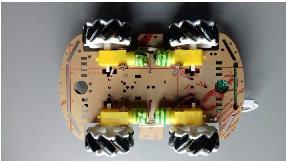
Note that where the red and blue wires attach to the motors, there is green and yellow masking tape to prevent any shorting and to ensure that the wires are held firm against the motors. The terminals on this make of motor are quite delicate and care should be taken to avoid any unnecessary movement.
