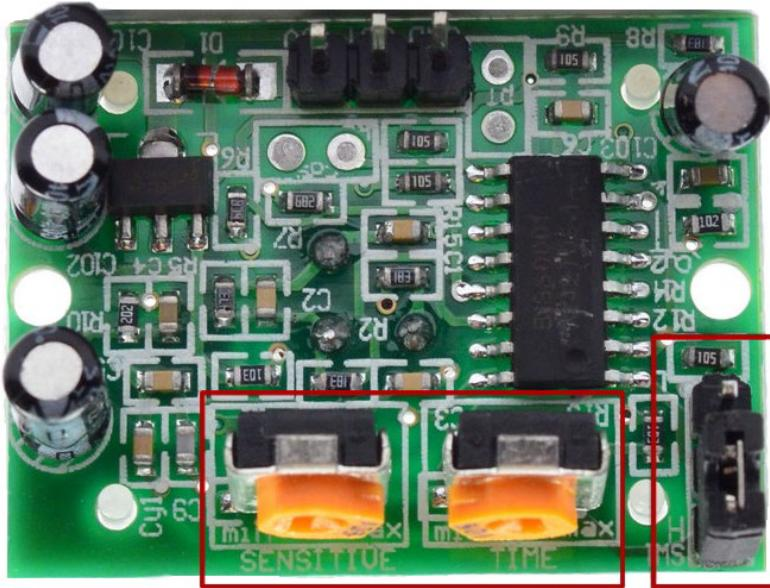
There are three possible adjustments of the motion sensor, two potentiometers and a jumper. All are on the bottom of the board, *i.e.*, the side opposite the lens and detector. You will need a small screwdriver to adjust the potentiometers.
