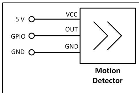
After you have determined which pin of the motion sensor is vcc, connect GND on the motion sensor to GND on the Raspberry Pi, OUT to a numbered GPIO pin, and Vcc to 5V. You will need to adjust your Python code to reflect the GPIO pin number you used; the example below uses GPIO 17.
