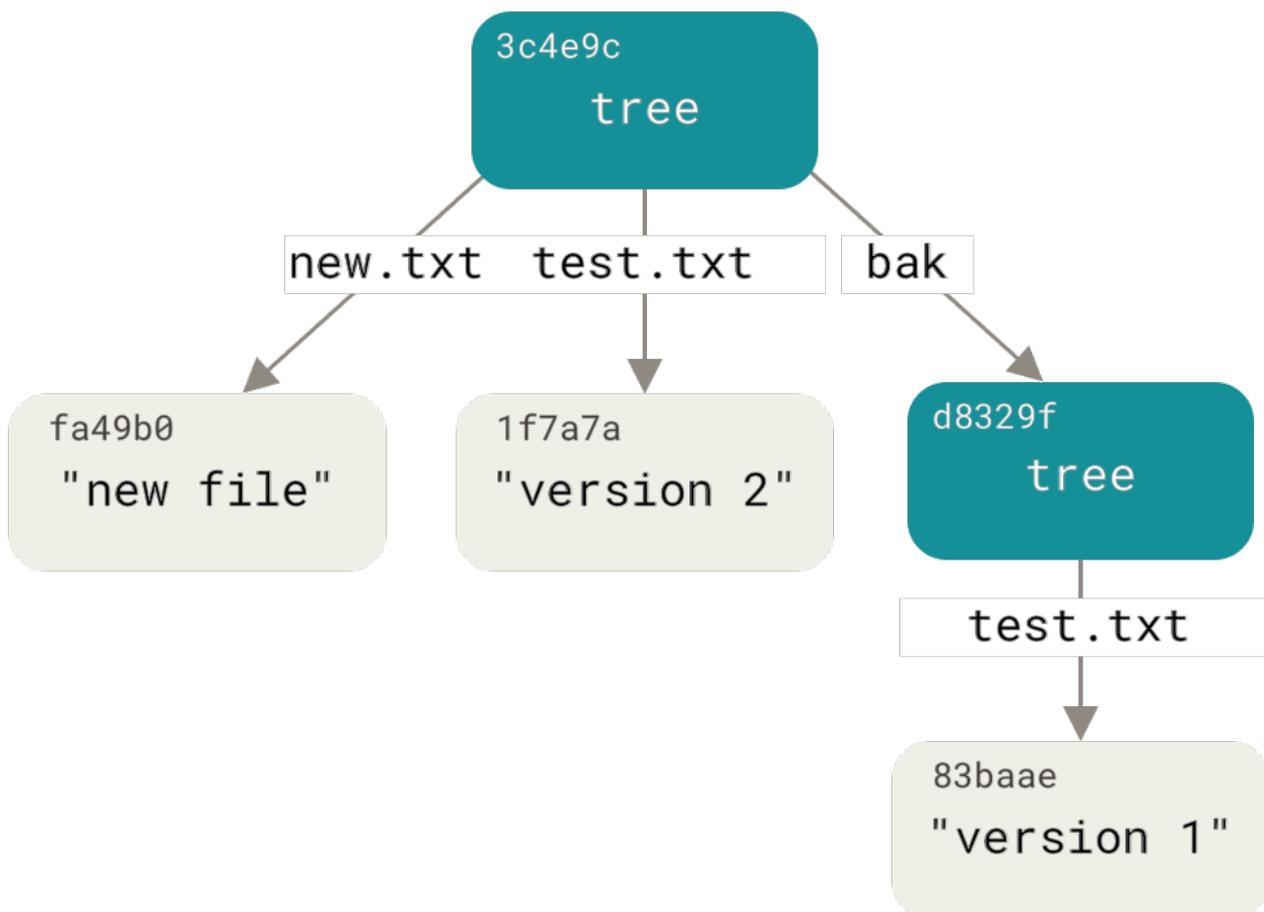
Figure 174. The content structure of your current Git data
