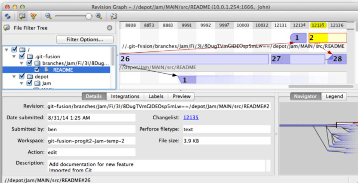
Figure 172. Perforce revision graph resulting from Git push
