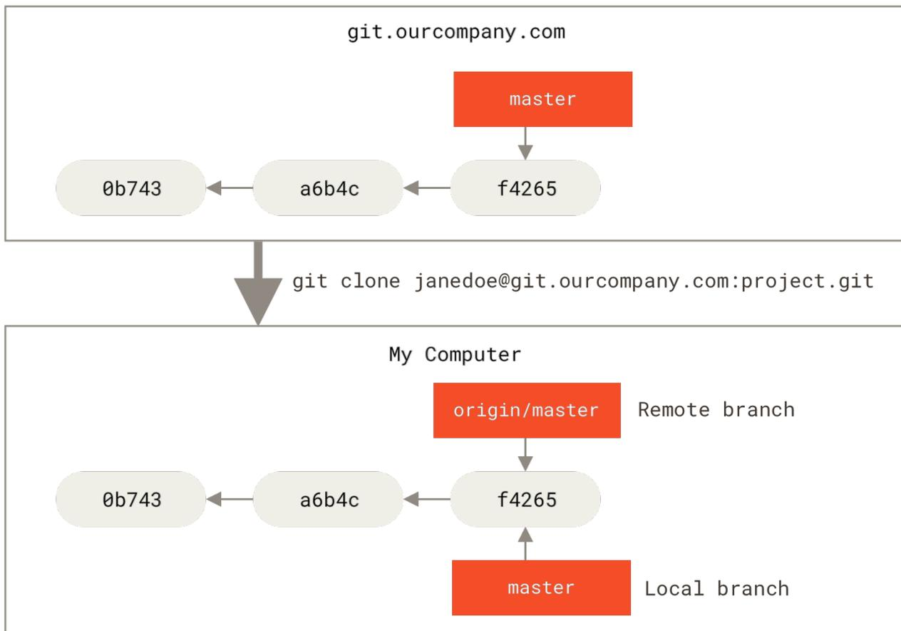
Figure 30. Server and local repositories after cloning
