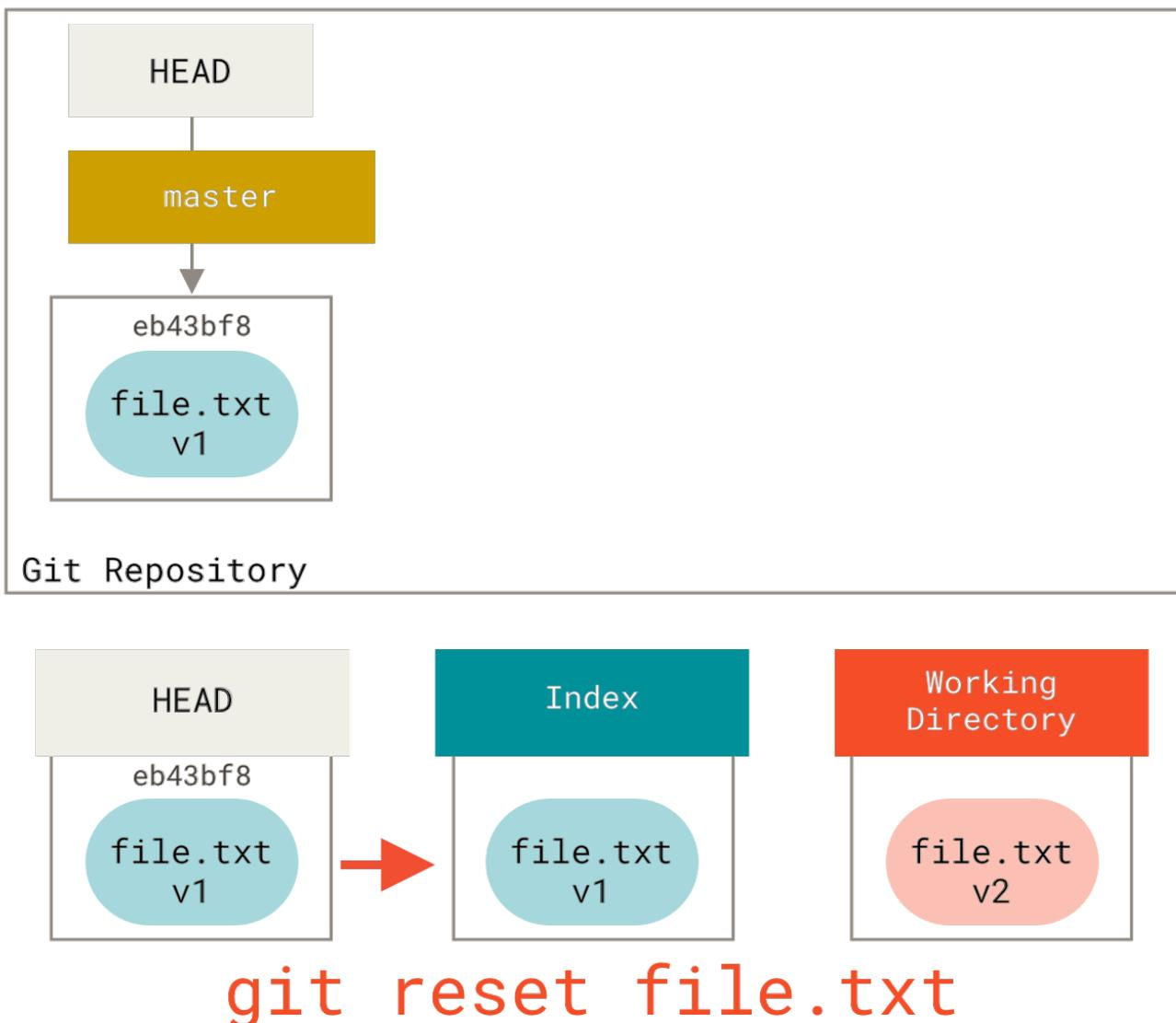
Figure 148. Mixed reset with a path
