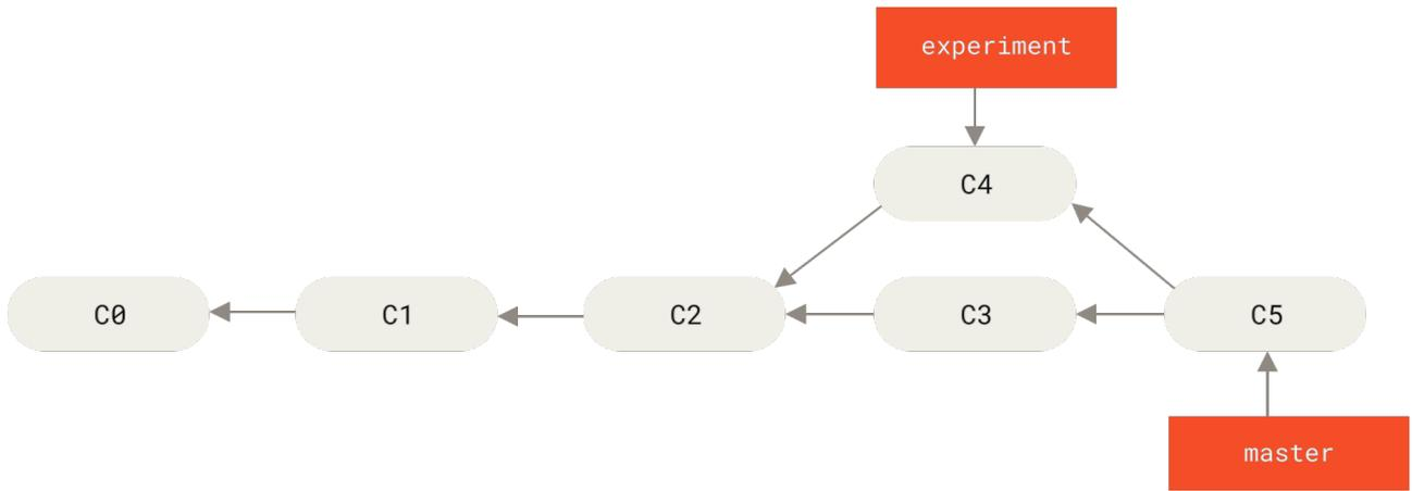
Figure 36. Merging to integrate diverged work history
