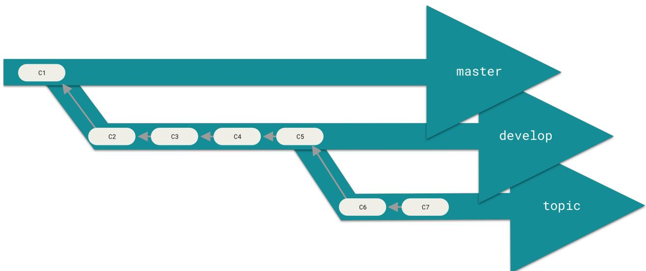
Figure 27. A “silo” view of progressive-stability branching
