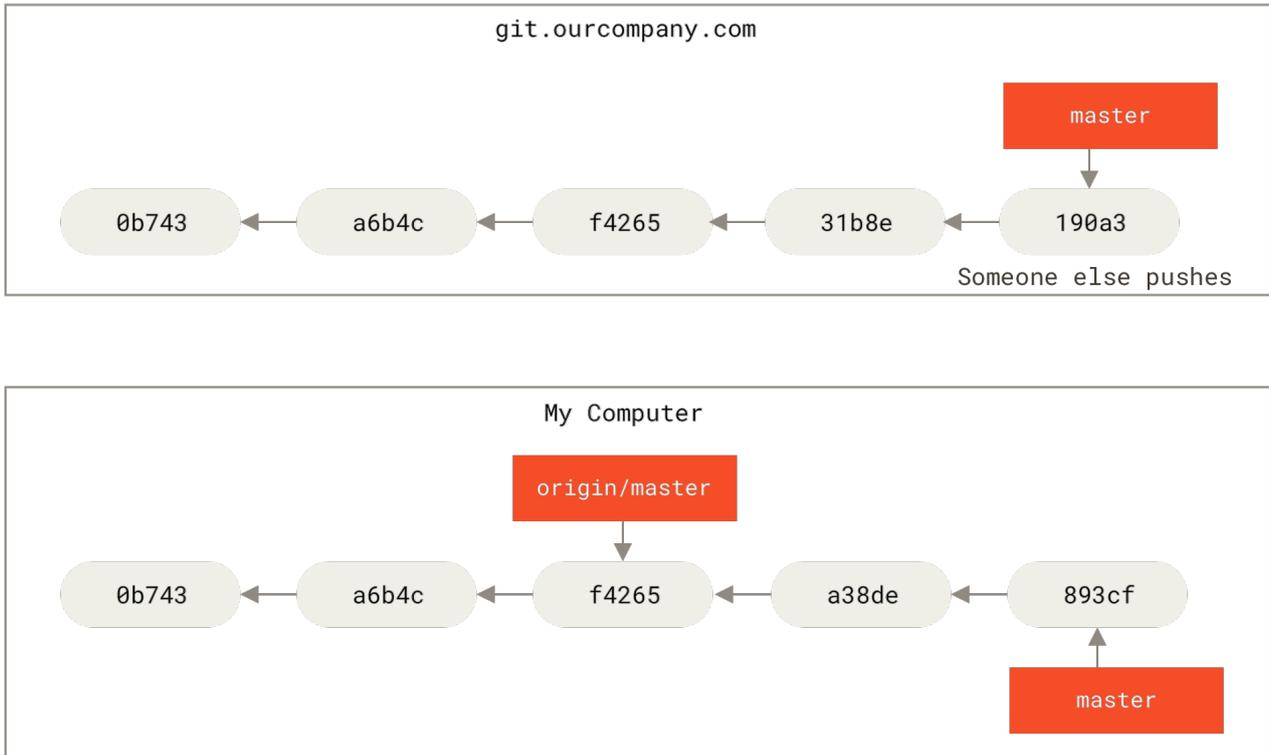
Figure 31. Local and remote work can diverge
