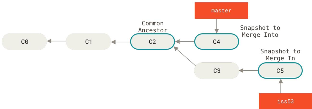
Figure 24. Three snapshots used in a typical merge
