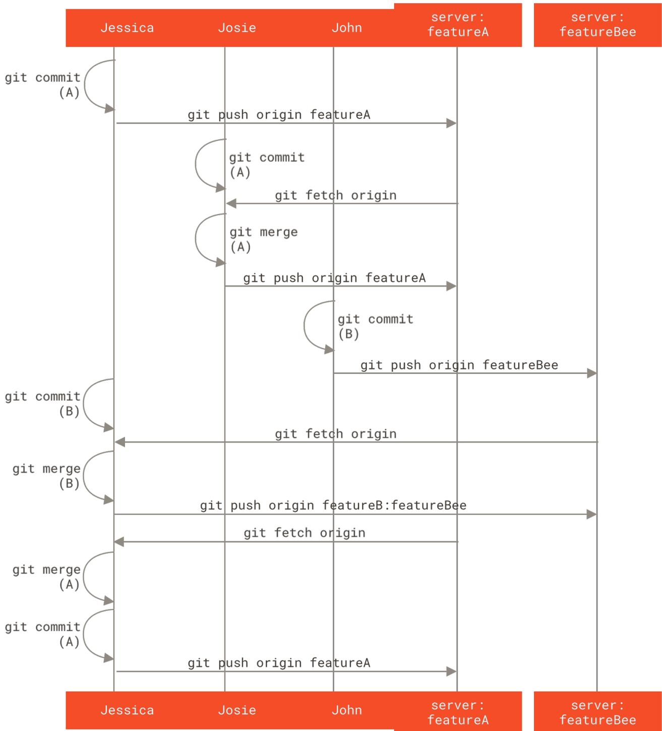
Figure 68. Basic sequence of this managed-team workflow
